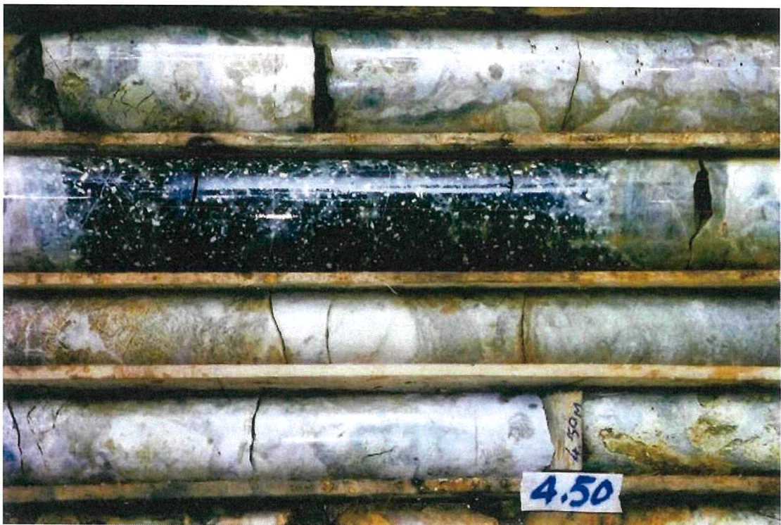
Figure 7. Drillhole BH3 shows Tsing Shan Monastery Plug. The dark green basaltic trachyandesite (chemical sample TM1 & TM104) intrudes the explosive breccia forming reaction rims. Lithic clasts consist of marble, sandstone and lava fragments, cemented by andesite
